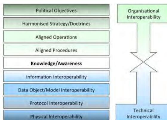
Fig. 3 Layers of interoperability according to ESENET.
